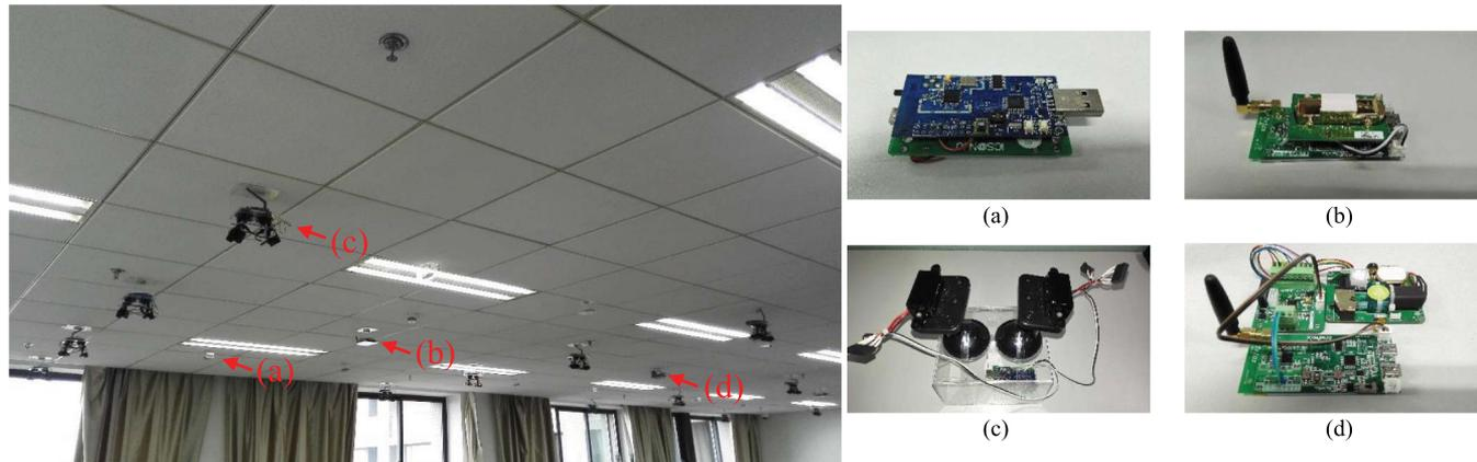
Fig. 20. Sensor network in the iLab application. (a) Temperature and light intensity sensor. (b) CO<sub>2</sub> sensor. (c) Active infrared sensor. (d) HCHO and PM<sub>2.5</sub> sensor.
