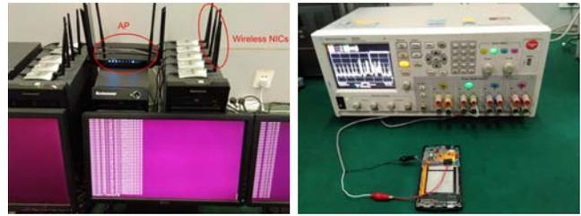
Fig. 7. left: testbed setup; right: Nexus 4 phone connected to power meter.
