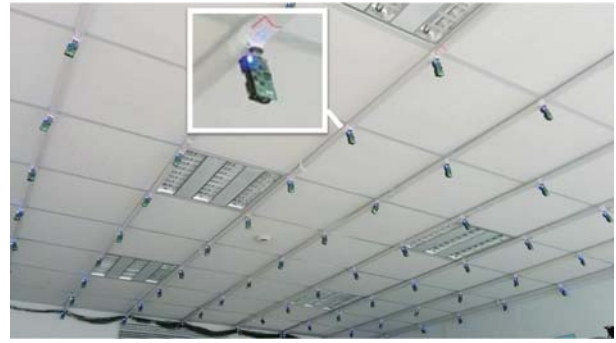
Fig. 7: The 8 \times 10 testbed with TelosB/TinyOS nodes.
