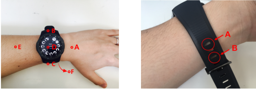
(a) The possible watch positions if wearing loosely: A is on the wrist (against the bone), B is outward slant, C is inward slant, D is the common snug wearing (close to wrist around 1cm), E is top of the wrist and F is facing down to hand
