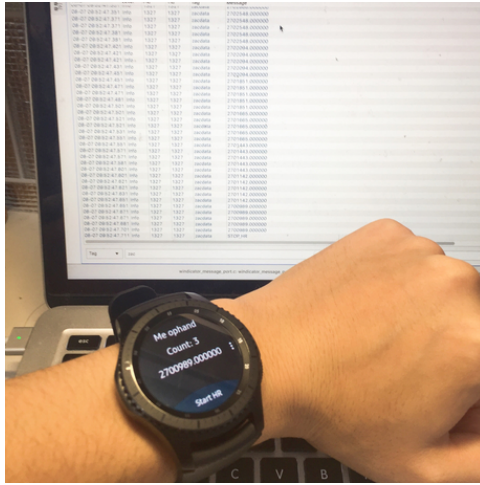
(a) An on-line data application implementation, which requires connection to a host computer for receiving data in real-time via TCP.
