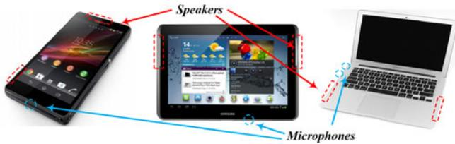
Fig. 2. Speakers and microphones in COTS mobile devices.
