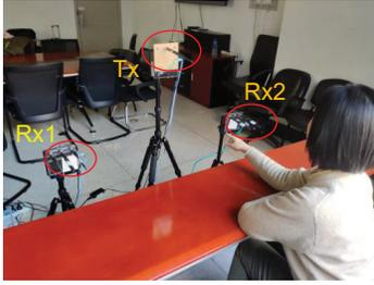
Fig. 18. illustration of the experimental setting in a meeting room
