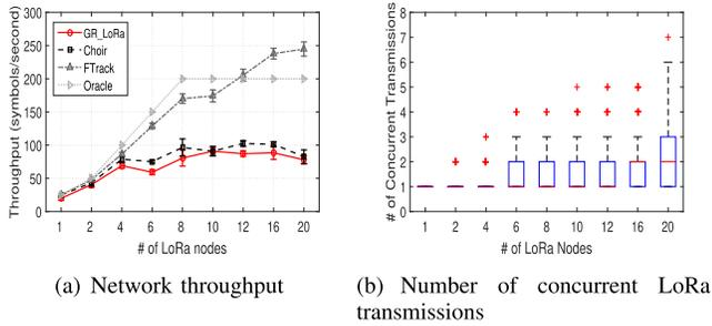
Fig. 23. Performance of decoding concurrent transmissions in real-world LoRaWAN network (SF=8, BW=250kHz).
