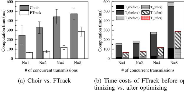
Fig. 21. Computational time of collision resolving with various number of concurrent transmissions: (a) The overall time costs (in milliseconds), (b) Anatomy of the time costs of FTrack:  $T_1$ —time of frequency track extraction,  $T_2$ —frame identification (preamble & symbol edge detecting) and  $T_0$ —others (including symbol classifying & iterative frame demodulation).
