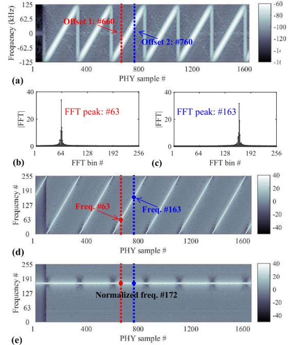
Fig. 11. Steps of extracting frequency tracks: (a) spectrogram of received signals (the preamble part), (b-c) dechirp the signal in *PHY Win* (FFT of dechirped signals at #660 and #760), (d) slide *PHY Win* across all samples (the frequency of dechirped signal vs. offsets of *PHY Win*), (e) remove the frequency deviation induced by  $t_w$  (*i.e.*, the time offset of *PHY Win*) to produce the normalized frequency of LoRa chirps, *i.e.*, frequency tracks.
