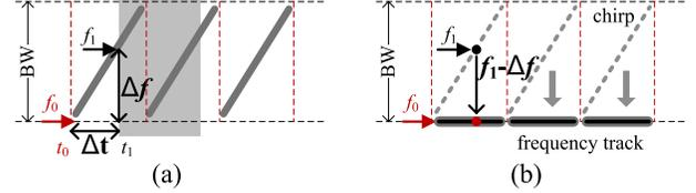
Fig. 3. Illustration of (a) preamble chirps, and (b) the corresponding frequency tracks, *i.e.*, normalize instantaneous frequency into the meta initial frequency.
