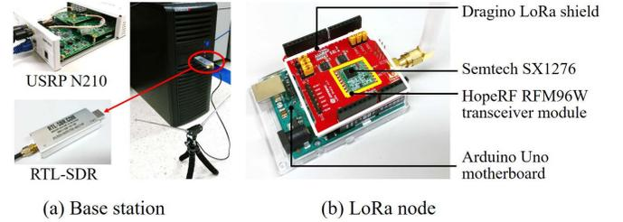
Fig. 14. Experiment equipment.
