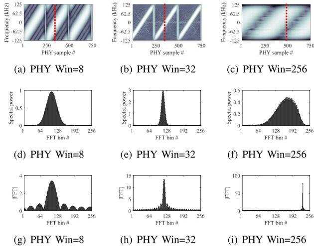
Fig. 9. Frequency estimation with different *PHY Wins* (the *FFT Win* is 256). (a-c): Spectrogram of preamble chirps; (d-f): Width of the FFT peak of original signal; (g-i): Width of the FFT peak of dechirped signal.
