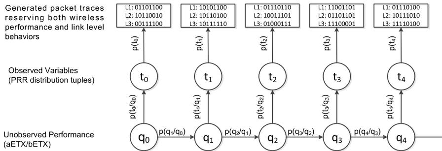
Fig. 3. The PA-HMM. The unobserved  $q$  states capture the performance state transitions (with aETX and bETX). The observed  $t$  states capture the link level behavior transitions (with PRR tuples, where a tuple indicates the PRR distribution at multiple receivers).
