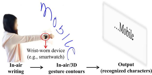
Fig. 1. AirContour: in-air writing gesture recognition based on contours.
