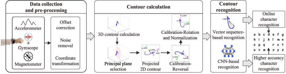
Fig. 16. Components and workflow of AirContour.
