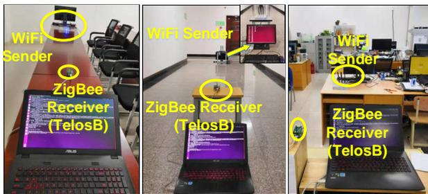
Figure 12: Experimental deployment from left to right, mildly interference meeting room, moderately interference corridor, severely interference lab.
