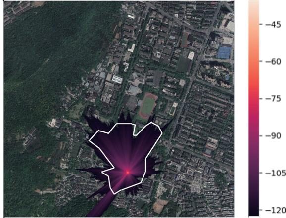
Fig. 12. Effectiveness of the ESP map of Yuquan Campus, Zhejiang University. The white lines show the measured signal coverage boundary.
